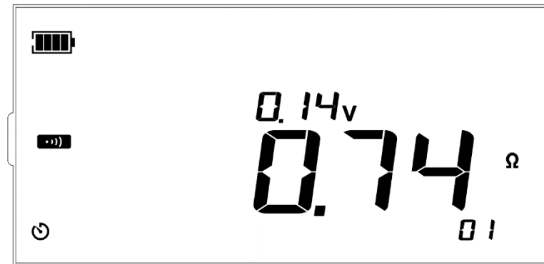
Figure 13.16 Test leads are shorted
