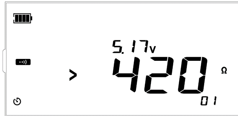
Figure 13.19 Low resistance exceeds the range
