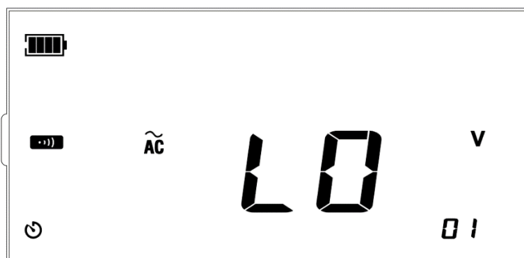
Figure 13.11 Voltage measurement (Default interface)
